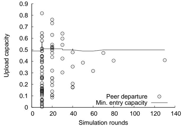
**Figure 6: Order of exit from a PropShare stream. Average capacity is 0.75.**
