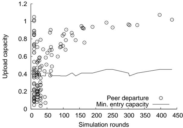
**Figure 5: Order of departure from a stream of BitTorrent clients. Average capacity is 0.75**
