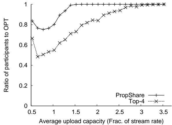
Figure 4: Number of system participants compared to the maximal amount from Algorithm 1.
